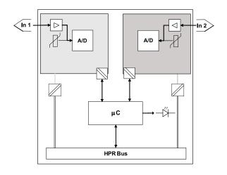
The TC-input module HE 5841 acquires up to two analogue measured values from thermocouples and transmits these to the higher-level bus system. The communication with the bus coupler takes place over an asynchronous serial RS-485 connection. In the event of service, the module can be exchanged quickly and without complications in running operation (Hot Swap). In addition a cold junction compensation with a constant value or with measured cold junction can be connected. The signal status of
