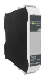
The power module HE 5850 offers a supplementary power supply of additional HIMOD modules. With the HIMOD power module, a connection of up to 62 modules per field bus coupler is possible, whereby each power module can supply up to 16 modules on a separate rail. The communication with the field bus coupler is maintained with a serial bus extension. The use of the power module enables a system expansion with distribution to various instal-
